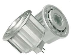
MR16 3W is designed for energy savings. It has a high light output efficiency but low power consumption. The stylish aluminum housing provides air ventilation to take away heat effectively. Temperature rise of the housing is less than 25 degrees and it is safe to touch.
